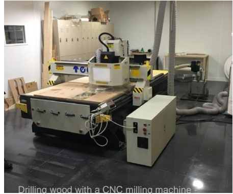
Drilling wood with a CNC milling machine → FabAcademy
